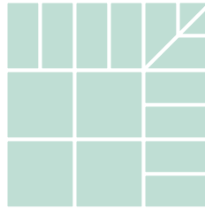
Corner-Cut 192 pcs. per 100 s/f 6" x 12" 96% 8 pcs. per 100 s/f 6" x 6" 4% (2 tiles are scored and cut to make corners)
